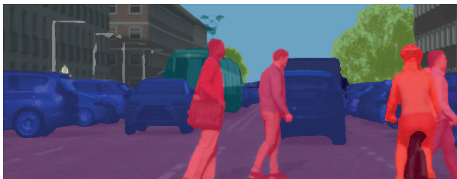
Figure 4.1: Example of aleatoric uncertainty in the task of street-scene semantic segmentation [85, 86]. Image pixels right at object boundaries are inherently more difficult to classify than pixels in the middle of objects.
